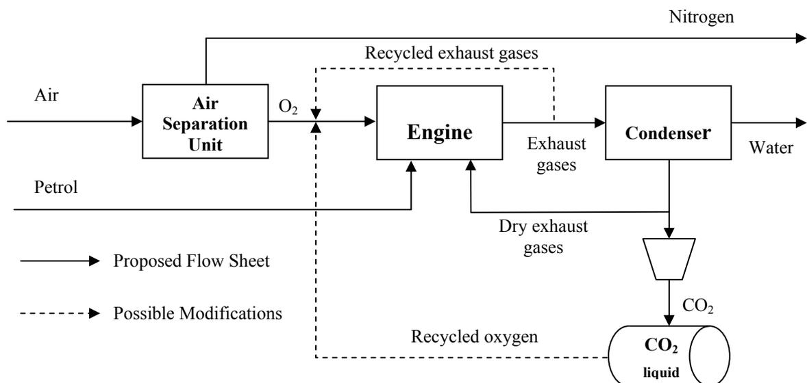
**Figure 1** – Schematic of closed cycle combustion for an ICE
