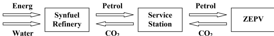
**Figure 2** – Schematic of carbon recycling in the transportation sector
